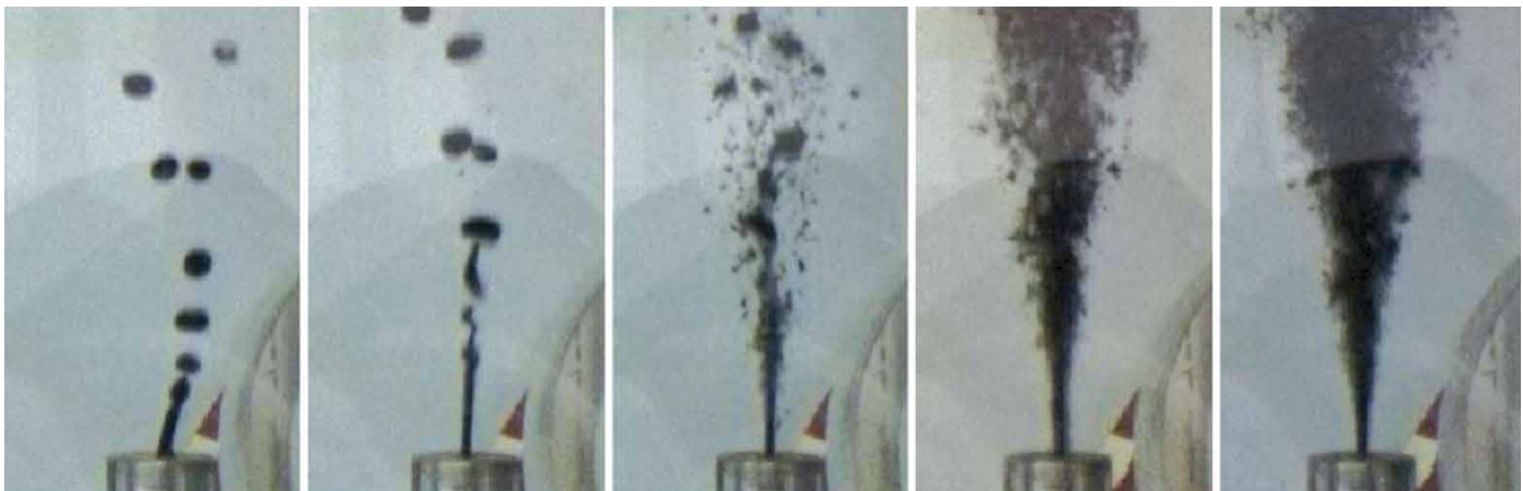
FIGURE 1. Oil droplets discharged into water through a 2 mm diameter nozzle (Tang and Masutani, 2003). From left to right, the jet exit velocities are 0.31, 0.97, 1.41, 2.42, and 5.99 m s -1 . As a point of reference, the nozzle outer diameter is 2.5 cm.
